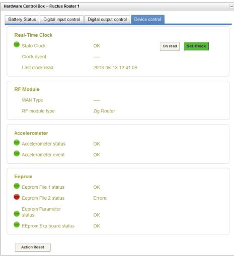
Fluctus Cloud Hardware Control Box allows the real-time check of Fluctus peripherals status, battery monitoring, reading and setting of Real Time Clock, control of digital inputs and outputs.
