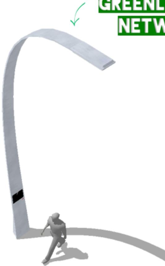
Consists in the **development of a network of street illumination devices**, based on LED technology and **wireless integrated modules** for network configuration, monitoring, providing multimedia and connectivity services.
